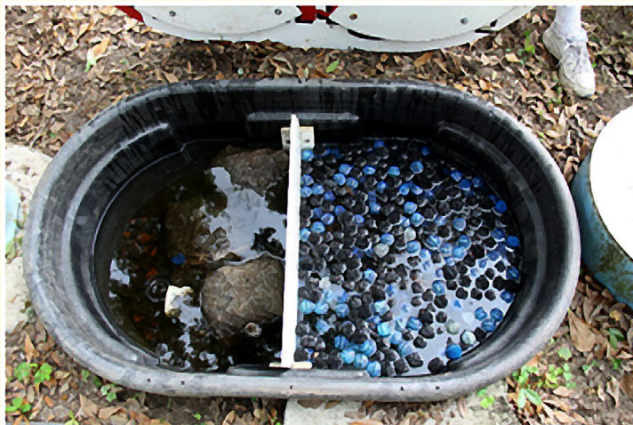
Photo 9: View into a filter. This one has bio-balls, lava rock, and shredded PVC.
