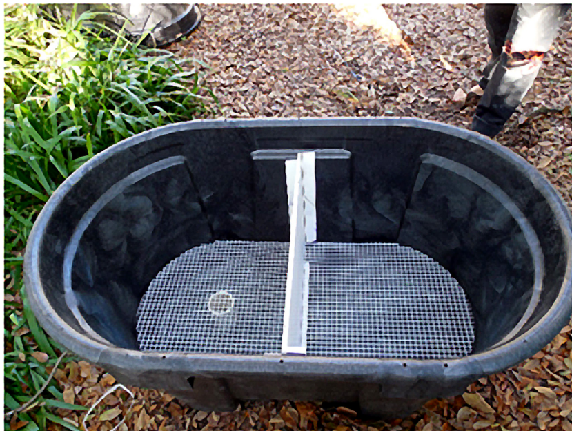
Photo 2: Tank showing divider & egg-crate bottom (one PVC support missing also no holes drilled).
