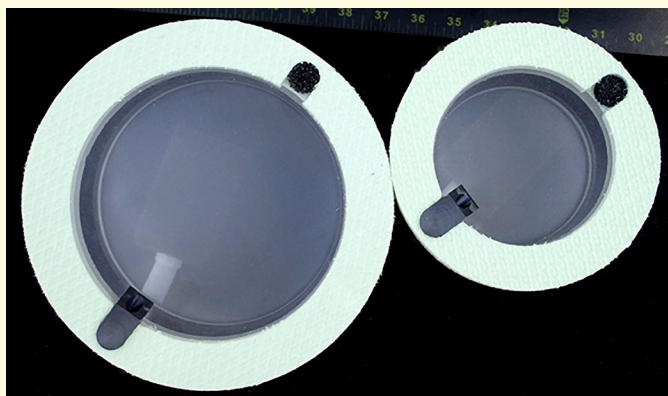
An overhead view of the large and small German Breeding Rings, showing the 30 micron mesh at the bottom of the chamber.
